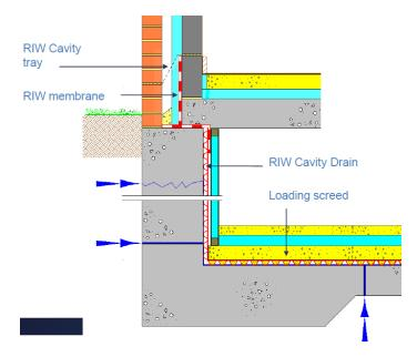
It is suitable for grades 2 and 3 with a high water table and requires a cavity drain with pump to collect and remove the water in order to minimises water ingress.
