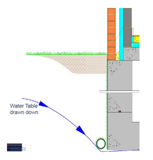
"During the life of the structure, some degree of groundwater pressure is likely to build up against the waterproofing system"\*
