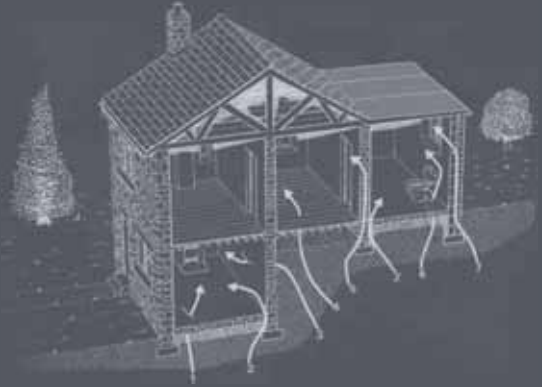
Figure 1 Routes by which radon enters a dwelling
