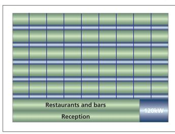
Hotel has 50 rooms. Each room has a cooling capacity of 3kW. The system is under the control of the hotel chain. The total under single control is 270kW, 150kW in the rooms and 120kW for the reception and restaurants. The system needs to be inspected by 4 Jan 2009.
