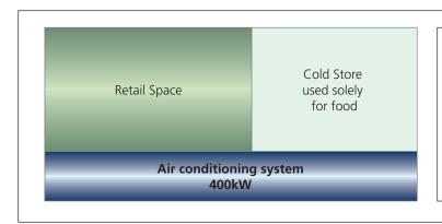
The retail space and cold store is served by a system under single control > 250kW. Even though the cold store is a process application, the airconditioning system also conditions space for the benefit of occupants in the retail space. The system needs to be inspected by 4 Jan 2009.
