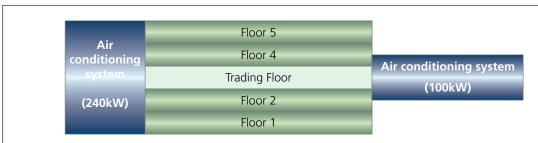
The building is served by a single system under single control < 250kW. In addition an air-conditioning system of 100kW has been installed to serve the trading floor. The total under single control is > 250kW. The system needs to be inspected by 4 Jan 2009.
